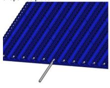
4. Make sure that the belt is not tensioned (tight) for any reason and includes catenary sag(s)
