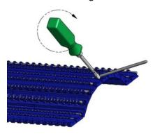
3. Separate the belt by pulling the lacing rod completely out.
