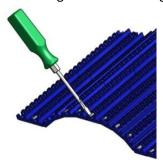
2. Turn the screwdriver clockwise so that the lacing rod lifts over the edge of the belt at an angle.
