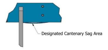
5. If needed, the catenary sag(s) can be adjusted by loosening the bolts, lifting the feed plate, repositioning and tightening the bolts on both sides of the conveyor.
