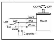
To rotate the motor in a clockwise (CW) direction, flip switch SW to CW.
