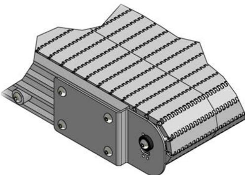
**Note:** If the ends overlap then remove the necessary number of links. “Punch” out a lacing rod (without a head on it) from the end.
