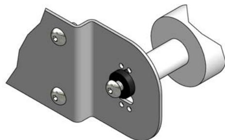
2. Line up adjustment space pins with holes in bracket. Tighten hardware and repeat for other side.
