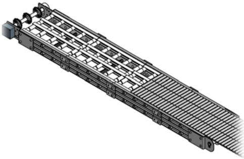
2. When the belt reaches the drive module make sure that the sprockets engage the belt correctly and wrap the belt around to the underside of the conveyor going over all the return rollers
