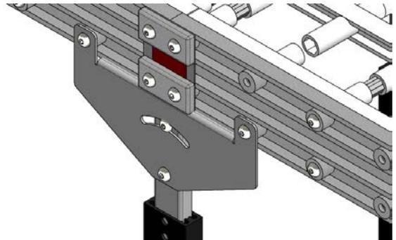
6. Adjust the height by removing the screws in the upright bracket and sliding the conveyor up or down to the desired height
