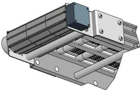
3. When the belt reaches the tail stock module bring the belting together so the ends interlock without much effort
