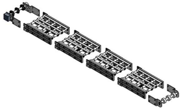
2. All DynaCon conveyors consist of a Drive Module, Feed Module and at least one (1) Mid Module
