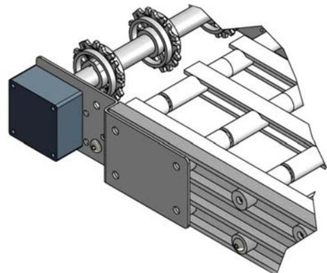
3. Add hardware to secure the drive module
