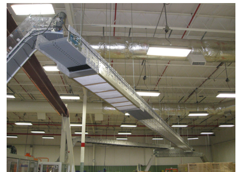
24" width ceiling hung filtered air conveyor system frees up floor space.
