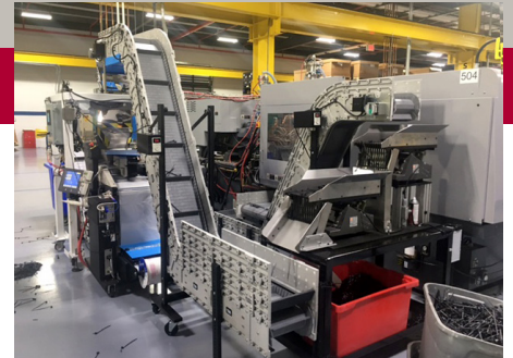
Modular conveyor with parts containment kit, chute & hopper and brushless high efficiency motor.
