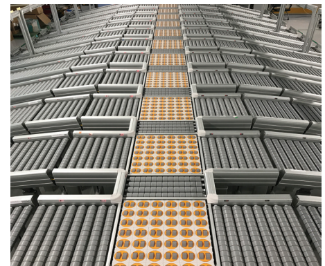
Multiple OTU for 20+ sort stations.
