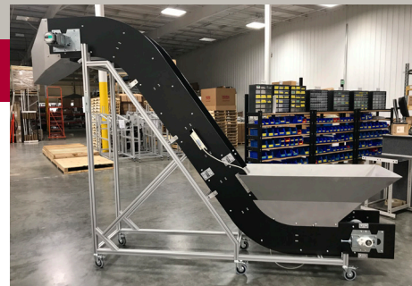
Large capacity stainless steel hopper that includes an integrated metal detection system.
