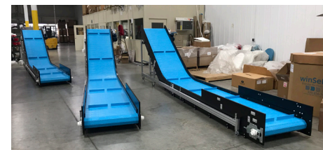
High impact belt with continuous side walls and abrasion resistance.
