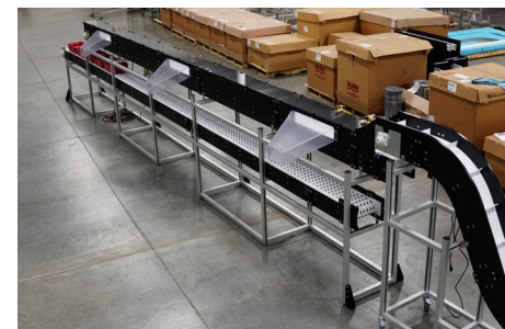
Multi-stack conveyor solution with three sort/divert stations.
