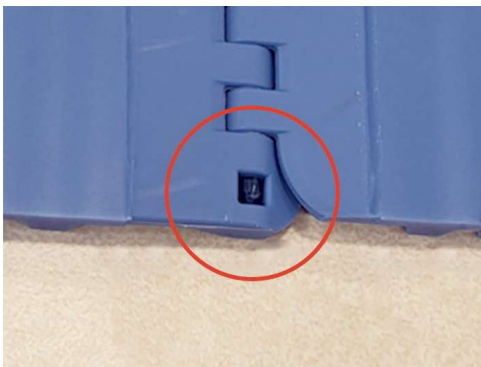
Figure 7: Ensure rod ends are visible in both viewing windows
