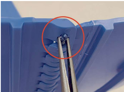
Figure 11: Use pliers to clamp rod
