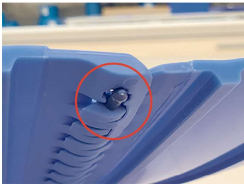
Figure 4: Ensure rod end stops \frac{1}{8} in from belt edge
