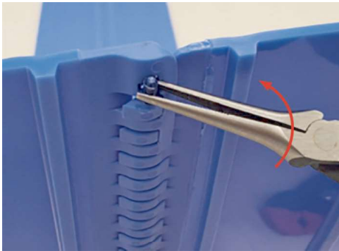
Figure 12: Twist pliers counterclockwise while maintaining pressure
