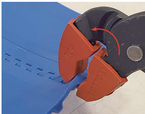
Figure 9: Flex belt edge upward to capture rod end
