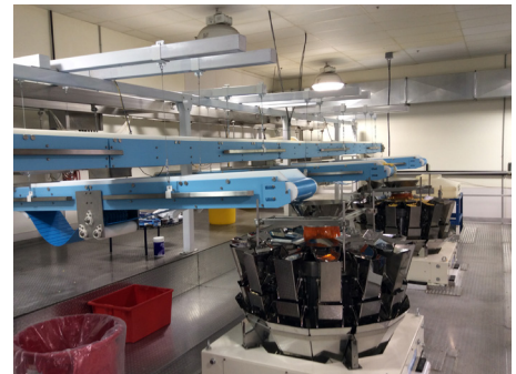
DynaClean® conveyors are ideal for food processing facilities. Constructed from a variety of plastic link style or ThermoDrive solid surface belting makes them easy to clean.
