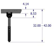
Adjustable leg height, bracket mounted option, floor mounted frame option.
