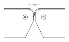
Distance between nosebar centers allows for tight transfer of products.
