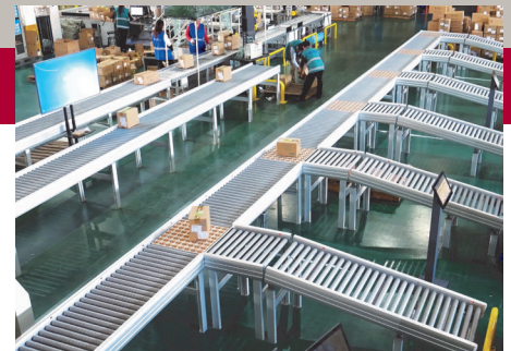
Large multi-station sortation handles a variety of parcel sizes.
