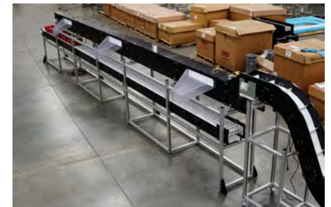
Multi-stack conveyor solution with three sort/divert stations.
