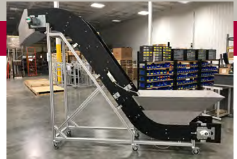
Large capacity stainless steel hopper that includes an integrated metal detection system.
