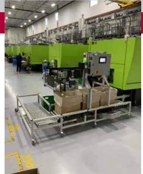
Inline configuration includes scale for weights and supports a lights out manufacturing strategy.
